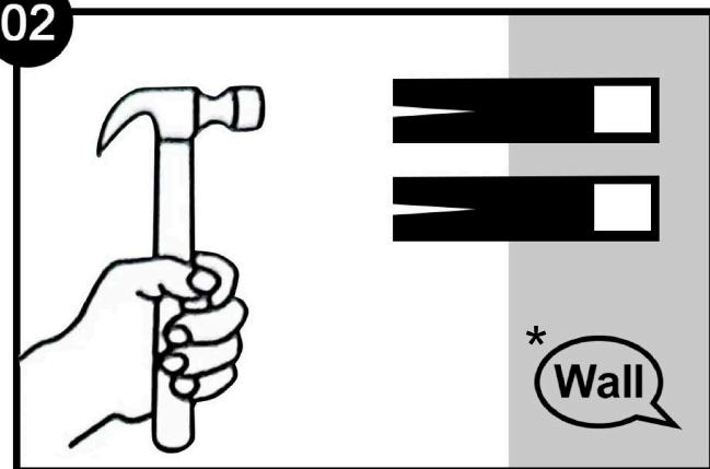
EN/ Using a hammer to insert the anchor onto the solid wall.
