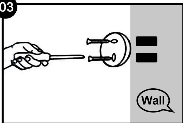
EN/ Putting the base plate over the anchor, then insert the screws with a screwdriver.
