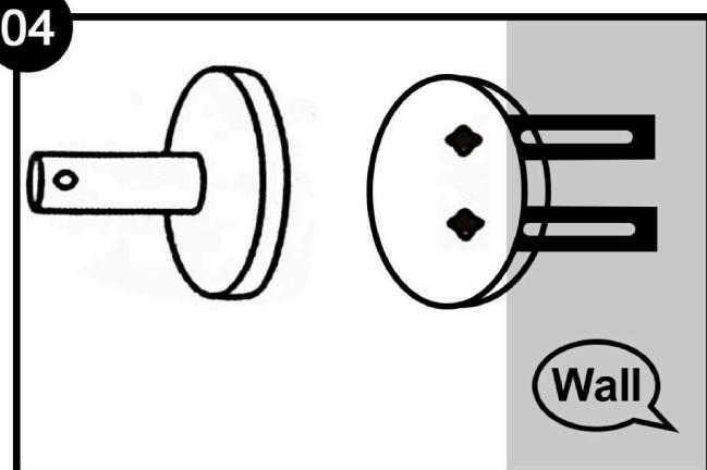
EN/ Attach the post onto the base plate.
