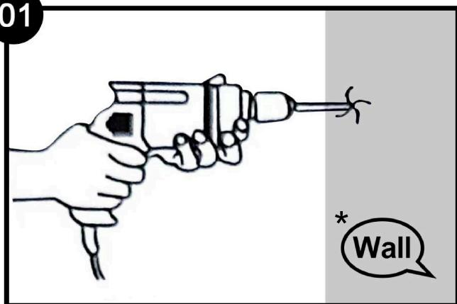
EN/ Drill the holes after measuring the location of installation holes.
